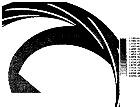
Fig. 6 Pressure distribution in impeller and diffuser of 380model for 36520 rpm, 2.39 m 3 /min
