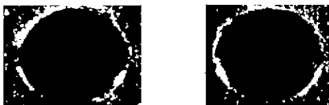
(1) 20,000rpm (2) 30,000rpm Fig.9 Comparison of micro hole form for a drill diameter 0.2mm(SM45C)
