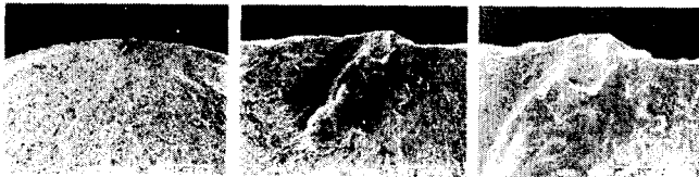
Fig. 18 SEM photographs of fracture surface around crack initiation point for specimen 50CrV4 under 2 stage shot-peened
