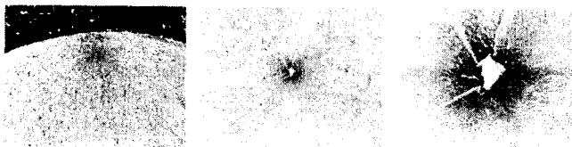
Fig. 19 SEM photographs of fish eye (nonmetal) fracture region under \Delta \sigma/2 = 160 kgf/mm 2
