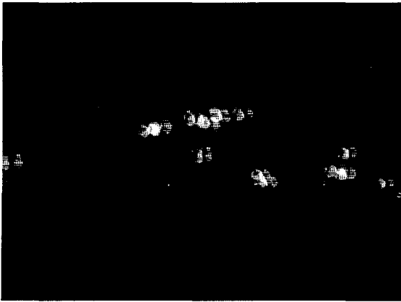
Fig.11 An Exemplified Raw Image Captured by CCD - Free Falling of Particles of Diameter 7mm
