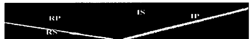
Fig. 5 Computed wavefield, showing reflected waves, for a mostly QP line source near free boundary
