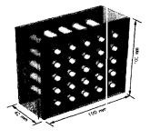
Fig. 1. Sand sediment container with water- and air- filled cylindrical pores of the radius 1.5 mm.
