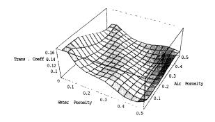
Fig.5. Theoretical 3D-plot of the transmission coefficient as the functions of water porosity and air porosity for the frequency 1 MHz.
