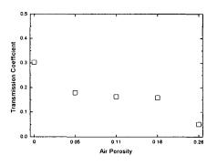
Fig. 4. Experimental transmission coefficient as a function of air porosity at the center frequency 1 MHz for air-filled sediment slab.
