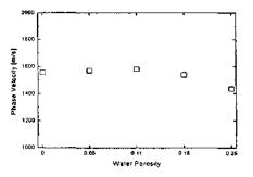
Fig. 3. Experimental phase velocity as a function of water porosity at the center frequency 1 MHz for water-filled sediment slab.
