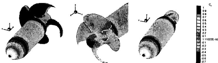
(b) Surface pressure distribution for Pusher type
