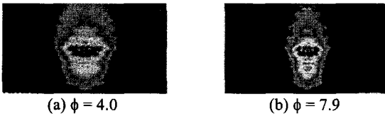
Fig. 8 Acetone PLIF image with primary combustion zone equivalence ratio change
