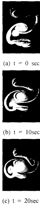
Fig. 4 LIF sequence of the columnar vortex in the cross-sectional plane as it interact with a clean free surface z=0.2 cm, Re=112 , Fr=0.12
