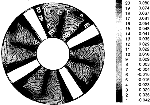
Fig. 14 Radial velocity in the blade( z=0.03 )
