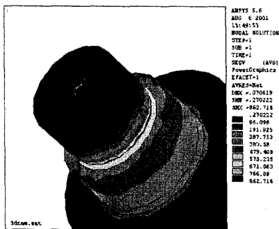
Fig.6 Stress distribution of cam
