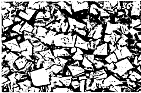
Fig. 3. SEM image of Diamond
