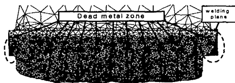
Fig. 5 Dead metal zone on welding plane
