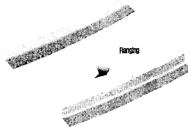
Fig. 6 Deformed shape of part model for flanging simulation
