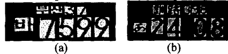
Fig. 7. Segmented Results of Korean and Japanese Vehicle License Plate; (a) Korean License Plate, (b) Japanese License Plate.
