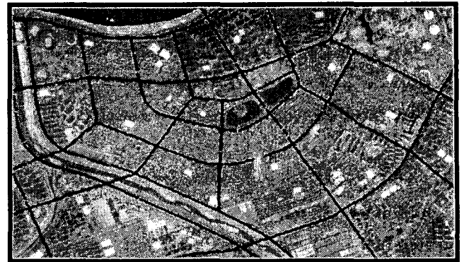
Figure 6. The result of road extraction on the dense metropolitan city of Seoul.
