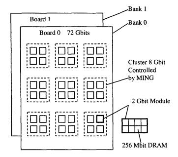
If there is a faulty cluster in a board, it's easily replaced with redundant cluster by "TC\_CONF\_MEM" command. If there is two faulty clusters in a board and no invalid cluster in the other board, one invalid cluster can be replaced with a redundant cluster on the other board. In the case of more than two clusters are invalid in a board, the board is no longer available.
