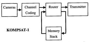
Due to output port to memory stack and to transmitter is separated in KOMPSAT-1, it's easy to perform real-time transmission and storage. All image data from cameras are first channel coded with CCSDS format and transmitted to transponder while same data is sending to memory stack.
