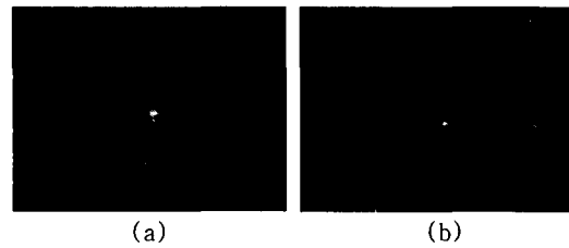
Fig. 7 Mode profile of the fabricated switch when the electrode is (a) unheated and (b) heated
