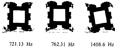
Fig. 5 First three mode shapes of stage with fine meshed finite element model
