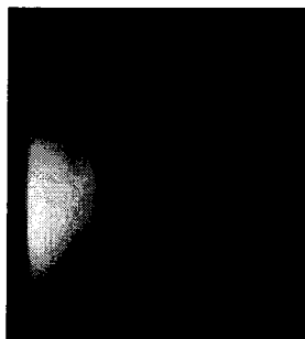
Fig.5 The X-ray irradiates on a fluorescent screen from left. The scanning conditions were the tube voltage at 120kV, the tube current at 250mA and scan time of 1s.
