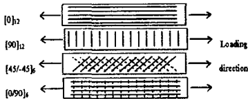
Fig. 2 Top view of tensile specimens with various raster angles.
