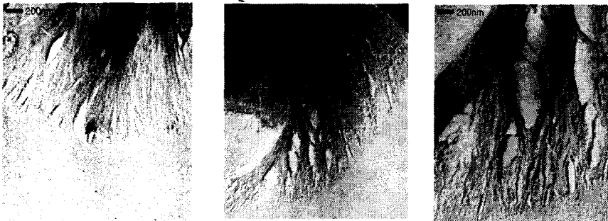
Figure 2. TEM images of Poly(ester-amide) with Degradation
