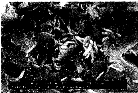
Fig. 5 SEM image of SG50-S concrete subjected to freeze-thaw action (90 cycles)
