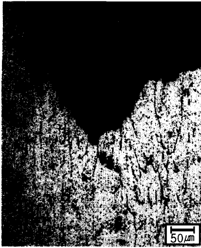
Fig. 2 Intergranular fracture at the tensile-fractured cross-section of as-cast Al6061 alloy.
