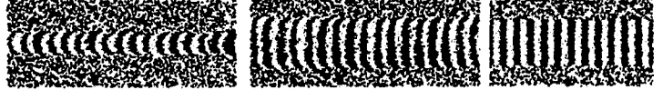
(i) ideal bit (ii) single layer (iii) double layer Fig. 1 Written bit pattern of three different cases (i) ideal bit in single layer, (ii) realistic bit in single layer without SUL, and (iii) realistic bit in double layer with SUL. Left hand is for the track width of 60 nm and right hand for 160nm.
