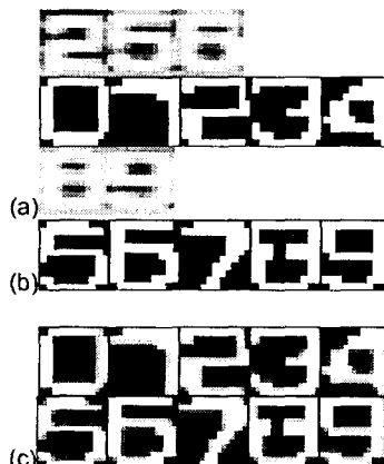
Figure 5. Examples of (a) original images in MBR, (b) enhanced binary images, and (c) mesh features.
