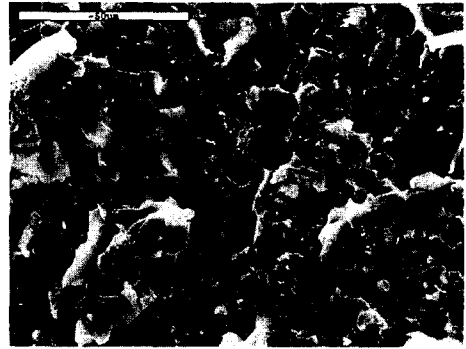
Fig. 5 The SEM photo of VGCF/Epoxy composite crack surface that contains 0.5 Vol%, made by simple mechanical mixing method
