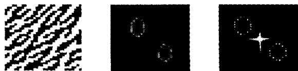
Fig.3. CGHs and its reconstructed image obtained using hybrid algorithm
