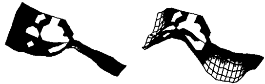
(a) Shape at 1.8 kHz (b) Shape at 2.5 kHz Fig. 7 Operational Deflection Shapes according to Peak Frequencies (Optical-Base)
