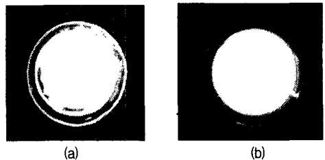
Fig. 18 Comparison of flame shape between (a) conventional swirler and (b) double cone premixed swirler
