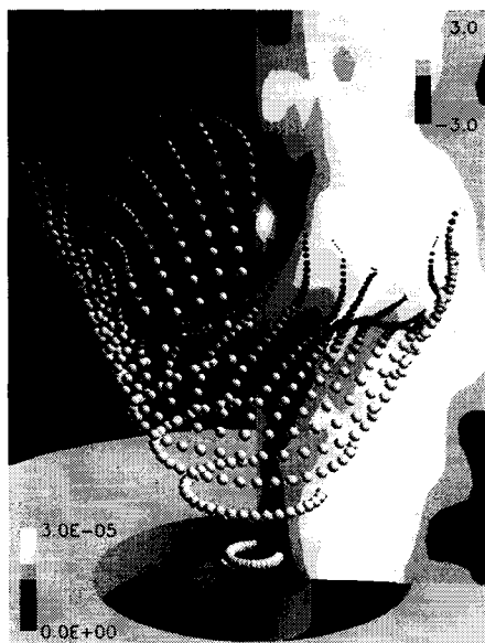
Figure 1: Typical instantaneous view of droplet motion and streamwise velocity contour plot
