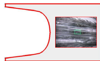
Fig. 5 Overload failure area
