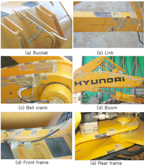
Fig. 3 Strain gages attached on a wheel loader
