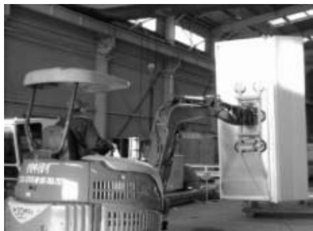
Fig. 3 Overturning test of a excavator
