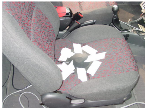
Fig. 3 Accelerometer for vibration measuring
