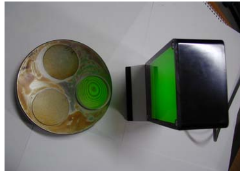
Fig. 9 The optical interference pattern of sapphire wafer
