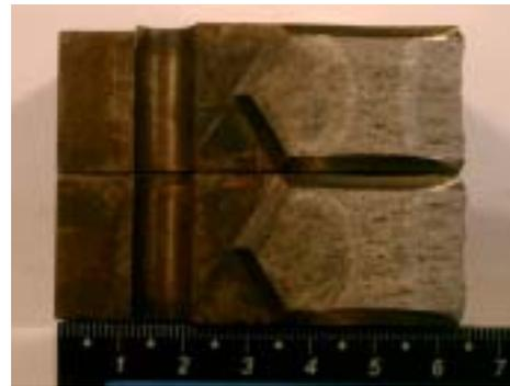
Fig. 4 CT specimen after J-R test
