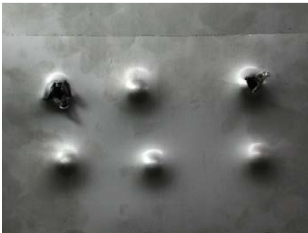
Fig. 12 PTP result of back face in Anodized Al(7plies) + Ti(8plies) laminates
