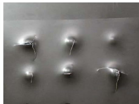
Fig. 10 PTP result of back face in Ti(8plies)/Anodized Al(7plies) laminates
