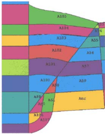
Fig. 14 Welding sequence of V-type model
