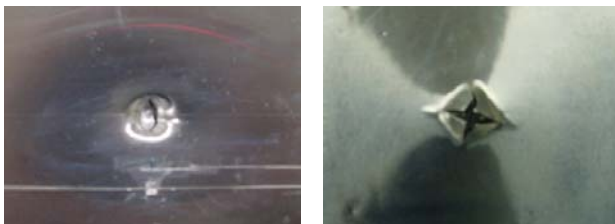
Fig. 8 (a)Front and (b)back face of FML[15/-15] at final failure
