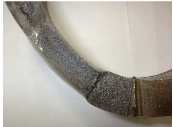
Fig. 7 Fracture appearance of pipe specimen
