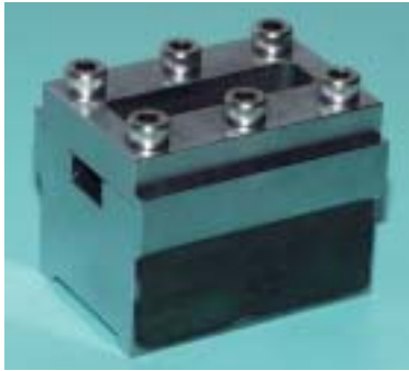
Fig. 7 Specimen fixture for the characteristic test of spacer grid spring.
