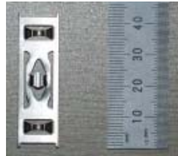
Fig. 5 Unit cell of optimized H-spring.
