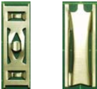
Fig. 8 Test Specimen of Springs (left: Opt. H; right: Doublet)
