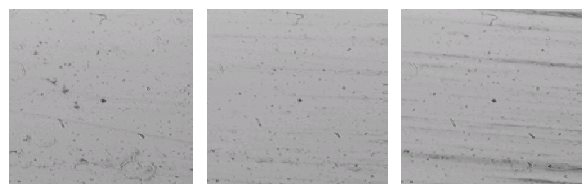
(a) Ra 0.2 μm (b) Ra 0.4 μm (c) Ra 0.8 μm
