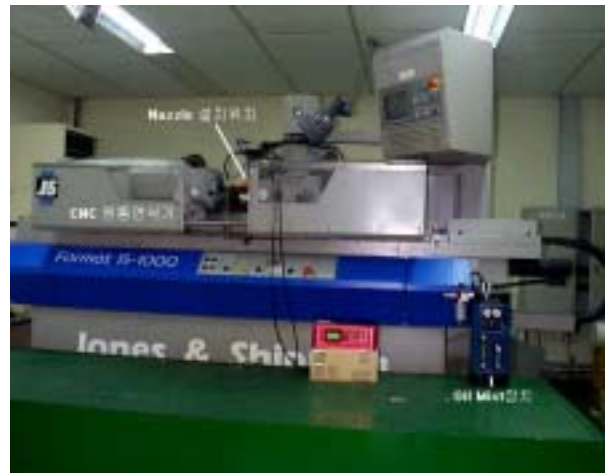
Fig. 2 Experimental Equipment for Cylindrical Grinding
