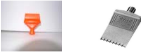
(a) Oil Mist Nozzle (b) Cold Air Nozzle Fig. 3 Photographs of Spray Type Nozzle
