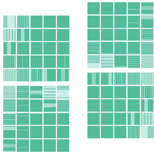
Fig. 3 The designed pattern with 100~1,000 nm line widths.
