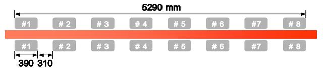
Fig. 3 Diagram of induction heater
