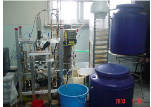
Fig. 3 Photograph of a lab-scale fouling experimental apparatus
