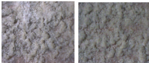
Fig. 10 Time history microphotographs at inlet temperature of 20 and velocity of 1.5m/s (magnification =100×)
