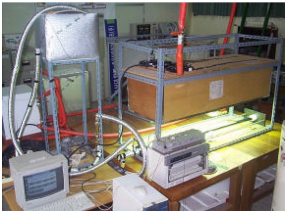
Fig. 2 Photograph of the experimental apparatus of one module evacuated solar collector.
