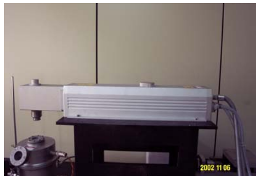
Fig. 3 Head.unit of Nd-Yag laser
