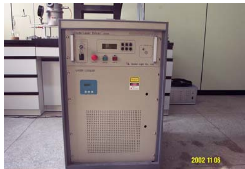
Fig. 2 Power supply and cooling unit
