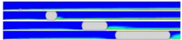
Fig. 5 Liquid temperature contours in a channel with H=1\text{mm} , \varphi = 40^\circ and \overline{u_{in}} = 0.16\text{m/s}
